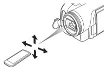
◆The distance between the remote control and the Camcorder: Within approx. 5 m (16 feet) Angle: Approx. 10° up and 15° down, left, and right
